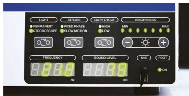
Frequency and sound pressure level are displayed on the stroboscope panel
